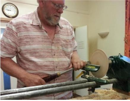
Now take the bowl off, mount the base on the chuck and start working on the top side.
