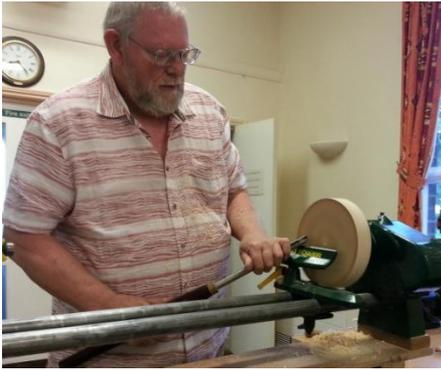
When the edge is trued up, move the toolrest round to the base. Make sure it's square to the wood to make the cuts easier.
